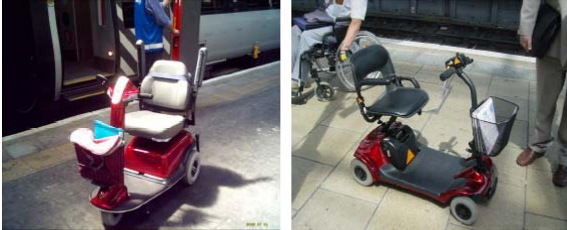
6.3.14 The trials highlighted very few problems with boarding, manoeuvring (as shown in picture below) and accommodating the small four-wheeler, which was tested on the Pendolino, Voyager and Class 158 and 175 units.
